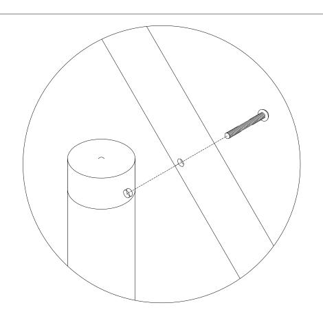
STEP 3: ATTACH RAILING (PN40015) TO BALUSTERS BY PASSING 2" BUTTON HEAD SOCKET CAP SCREWS (PN00922) THROUGH RAILING INTO TAPPED HOLES IN BALUSTERS
